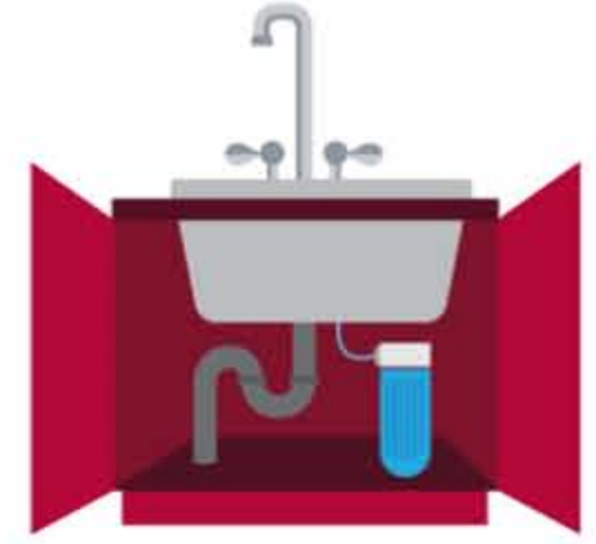
Under-the-counter water filtration unit
