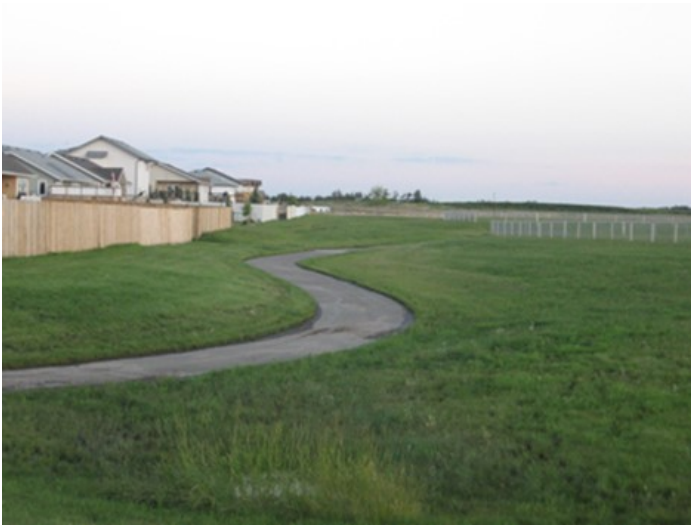
Pathways serve as walkways and storm water channels
